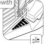
To prevent grass damage do not remove more than one third of grass height in one cut.
